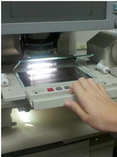
Pull out the guide until the two pieces of glass separate.
