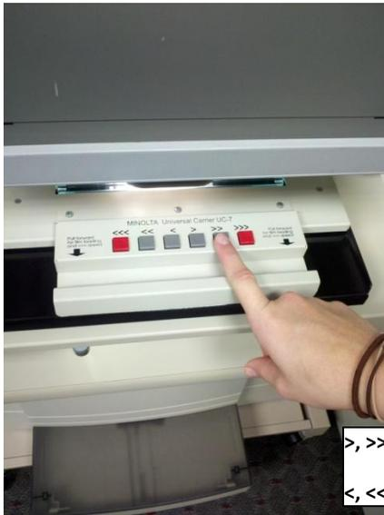
Use the colored buttons on the tray to scroll through the film. There are three scrolling speeds for moving through the film: slow, medium, and fast.
