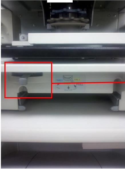
Pull out the lever below the fiche tray, called the brightness selector. Adjust to the appropriate position for the type of lens that has been loaded. The lever will click into position when it is set.
