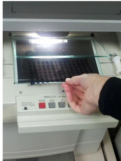
Place the fiche facedown under the glass and push the guide back under the lens.
