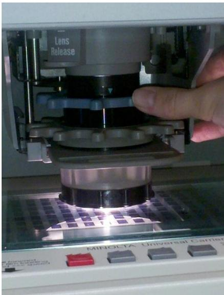
Move the blue dial clockwise (left) to reduce magnification, and counterclockwise (right) to increase magnification. Turn the blue dial to adjust sharpness.
